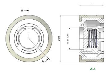
Non return valve Type DTEF for installation between flanges according to the correspondent drawings.
